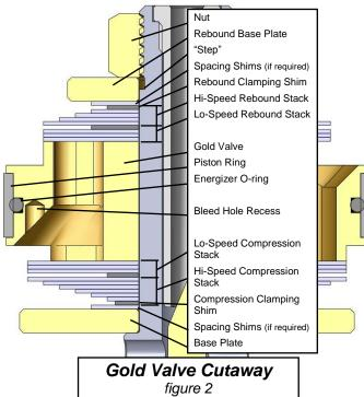
\* To add to the thickness of the valving stack you can use some of the original valving shims or <u>add flat</u> washers. Be sure the shims are <u>all</u> larger in diameter than the clamping shim (the last rebound shim, farthest away from the piston). If any of the shims or additional washers are smaller in diameter than the clamping shim it will decrease rebound damping. DO NOT PUT SHIMS BELOW THE COMPRESSION BASE PLATE!
